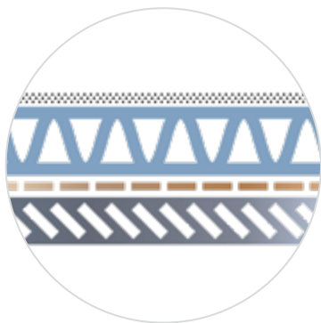
Three-layered sweatshirt fabric structure with a 100% cotton surface for optimal print results (Authentic Collection)
